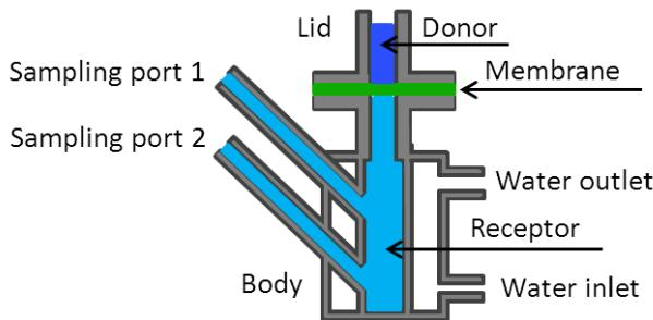
**Figure 2.** Schematic drawing of a Franz diffusion cell.
