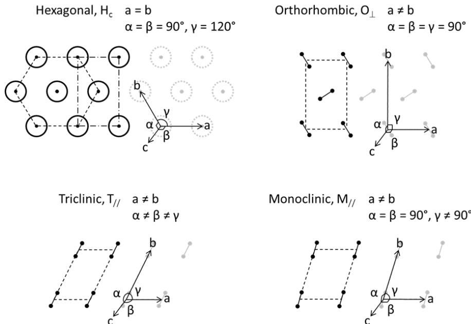
**Figure 5.** Short range order. Hexagonal, Orthorhombic, Triclinic, and Monoclinic sub cells.
